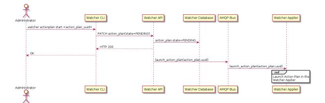
A message is sent on the AMQP bus which triggers the Action Plan in the Watcher Applier:
