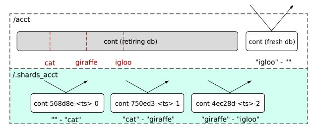
The sharder daemon cleaves objects from the retiring DB to the shard range DBs; it also moves any misplaced objects from the root containers fresh DB to the shard DB. Cleaving progress is represented by the blue line. Once the first shard range has been cleaved listing requests for that namespace are directed to the shard container. The root container still provides listings for the remainder of the namespace.
