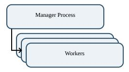
1. Manager process receives USR1 signal. This causes the process to fall out of its loop ensuring that all workers are running and instead begin reloading. The workers continue servicing client requests as long as their listen sockets remain open.
