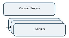
1. Manager process receives USR1 signal. This causes the process to fall out of its loop ensuring that all workers are running and instead begin reloading. The workers continue servicing client requests as long as their listen sockets remain open.
