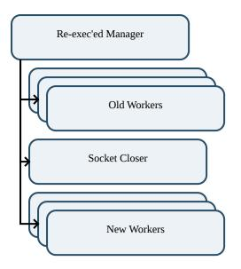
4. New manager process forks off new workers, each with its own listen socket. Once all workers have started and can accept new connections, the manager notifies the socket-closer via a pipe. The socket-closer closes the old worker listen sockets so they stop accepting new connections, passes the list of old workers to the new manager, then exits.
