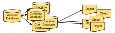
To keep track of object data locations, each account in the system has a database that references all of its containers, and each container database references each object.
