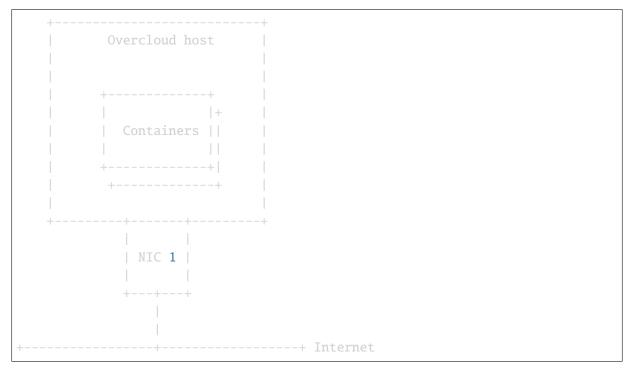
The networking in particular is relatively simple. The main interface of the overcloud host, labelled NIC 1 in the above diagram, will be used only for connectivity to the host and Internet access. A single Kayobe network called **aio** carries all control plane traffic, and is based on virtual networking that is local to the host.
