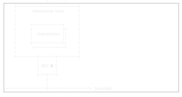
The networking in particular is relatively simple. The main interface of the overcloud host, labelled NIC 1 in the above diagram, will be used only for connectivity to the host and Internet access. A single Kayobe network called aio carries all control plane traffic, and is based on virtual networking that is local to the host.
