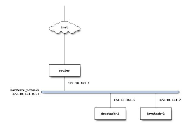
After DevStack installs and configures Neutron, traffic from guest VMs flows out of *devstack-2* (the compute node) and is encapsulated in a VXLAN tunnel back to *devstack-1* (the control node) where the L3 agent is running.
