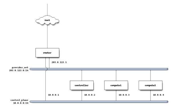
On a compute node, the first interface, eth0 is used for the OpenStack management (API, message bus, etc) as well as for ssh for an administrator to access the machine.
